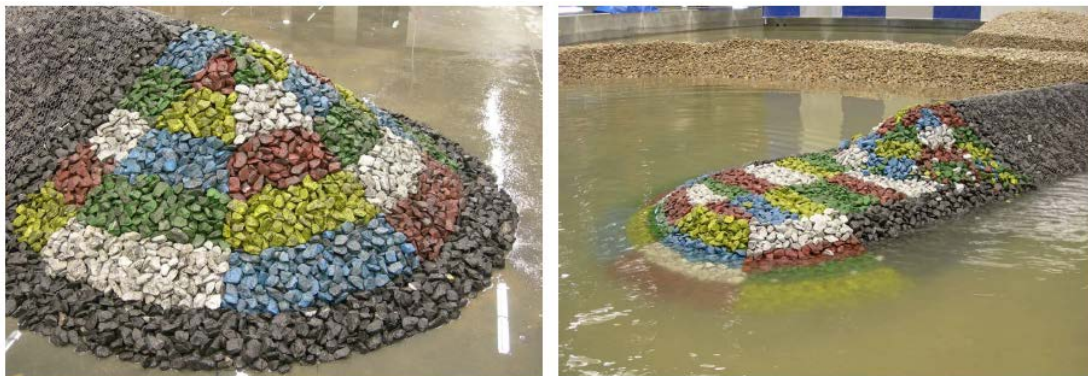
Figure 4 Left completed roundhead, Right temporary roundhead (Van Gent & Van der Werf, 2011)
