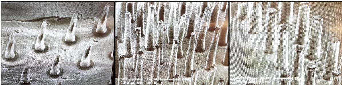
Figure 8 – Prototype 2 from left to right made with mask with circles with diameter of 20, 50 and 100 µm
