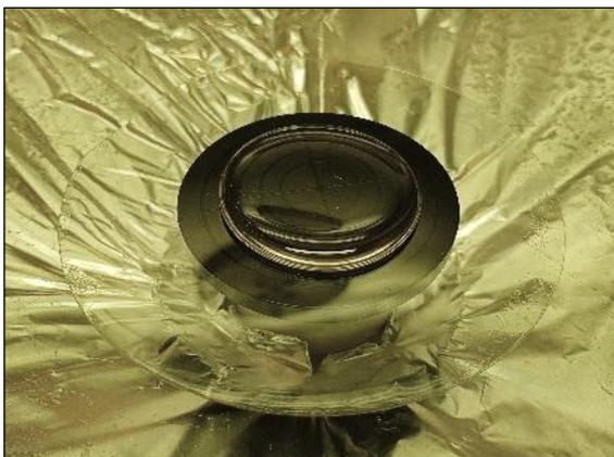
Figure 1 – A drop of SU-8 at the center of the wafer
