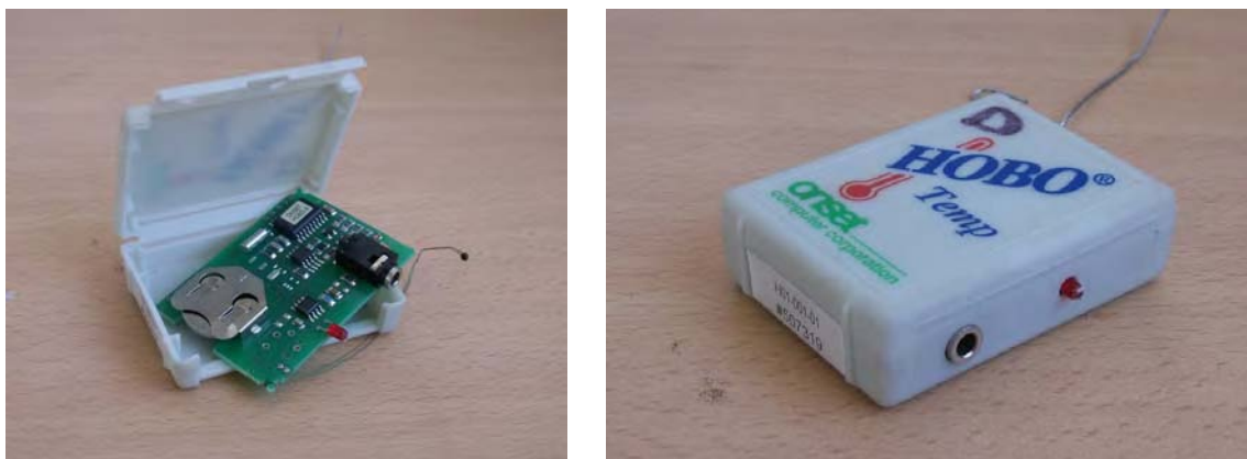
Figure 10.1. Miniature temperature data loggers, Onset HOBO, with the sensor and copper wire outside the box to obtain a rapid response to temperature variation.
