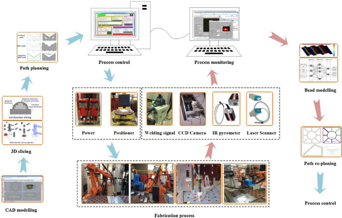
Figure 2.2 WAAM system design concepts [37].
