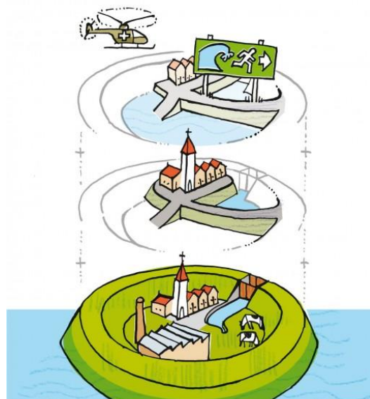
Figure 1-4 Multilayer safety. From top to bottom: crisis management, spatial planning/water robust design, prevention
