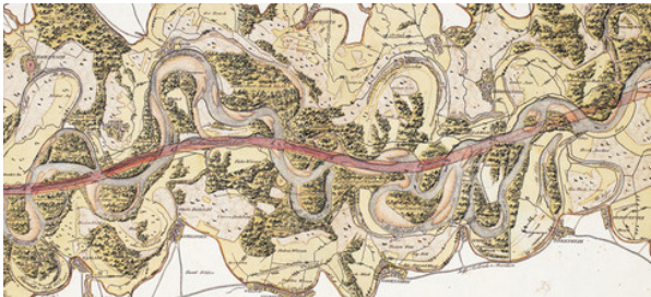
Transport Engineering works along the Rhine river adapted to it to a more controlled and efficient transportation route. In the map, the red line superposes the geological meanders of the river.
