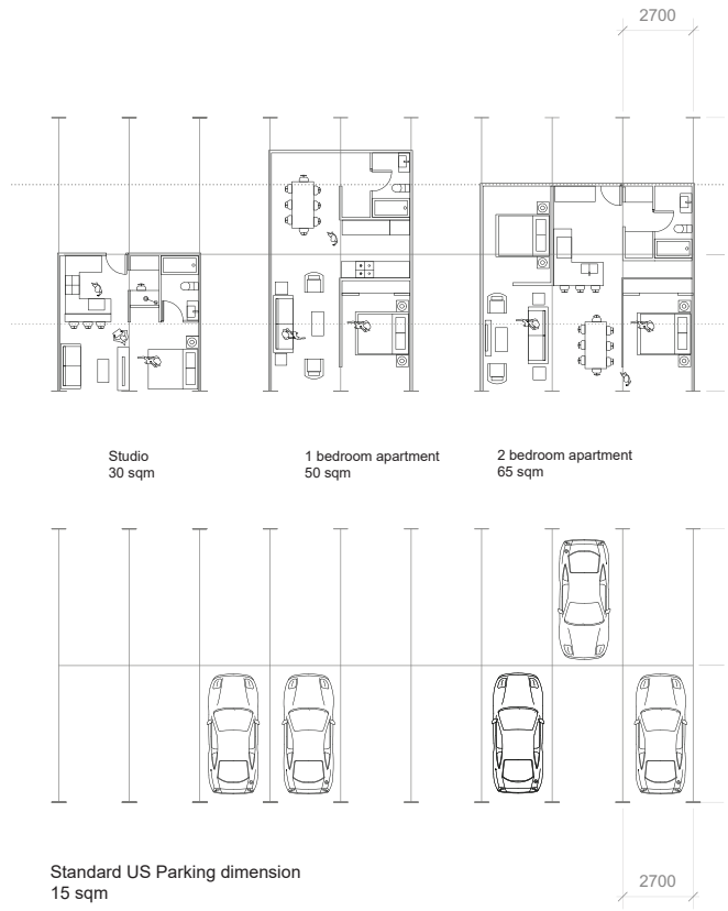
08.06.11 Converting Parking into usable area to meet housing demand. Parking space dimensions are easily adaptable to standard HPD/HDC affordable housing unit sizes.
