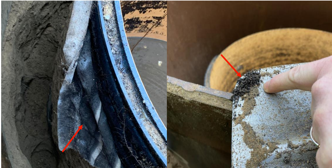
Figure 32: Traces of clogging around IDWs in Arnhem
