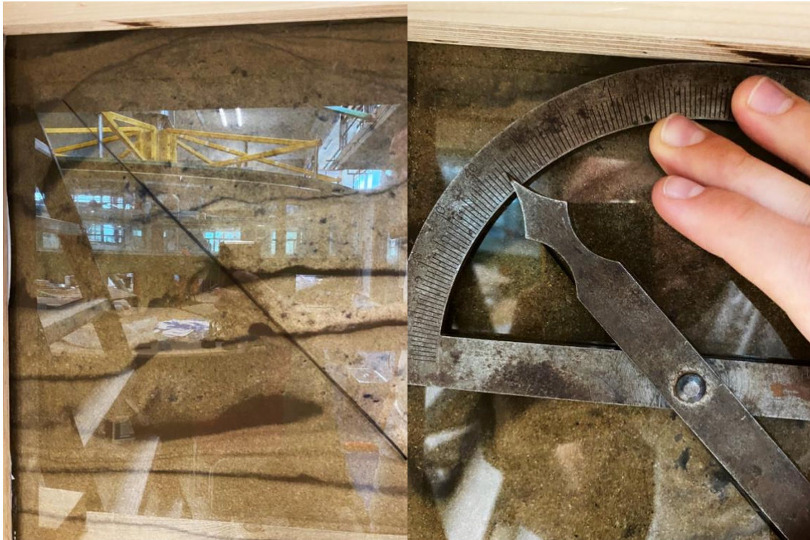
Figure 21: Images depicting the wetting front during the experiment, including a ruler indicating the angle
