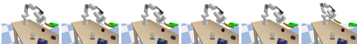
Figure 3.2: Failed generation of handover keyframes using a heuristic: 1) the joint-velocities are near zero, 2) the gripper open state has not changed
