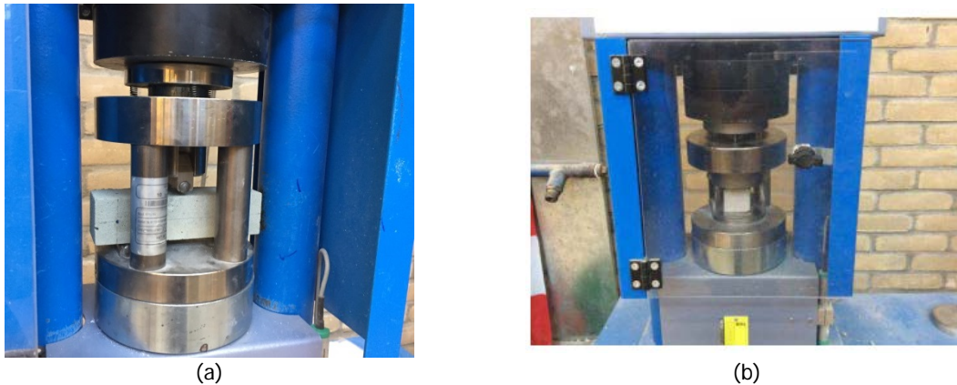
Figure 2 – Test on masonry mortar specimens: (a) three-point bending test; (b) compression test.
