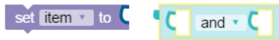
Figure 2: left is a block asking for input next to the block, right is a block asking for input inside the block. Both blocks are from open-Roberta [15].
