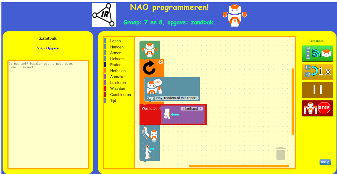
Figure 2: The exercise page for students. This page contains all the information for exercises and a workspace to do them in. It also contains start, step, pause and stop buttons to let the GOAL agent know to execute the program. The language is in Dutch because the user tests were conducted with Dutch children. The text is also not the focus here as the image serves to give an idea of the structure of the exercise page only.
