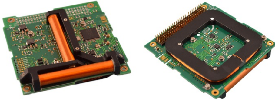
Figure 4.1: CubeSat magnetorquer board with flight heritage see; https://www.cubesatshop.com/product/isis-magnetorquer-board-retrieved(Nov 2018)
