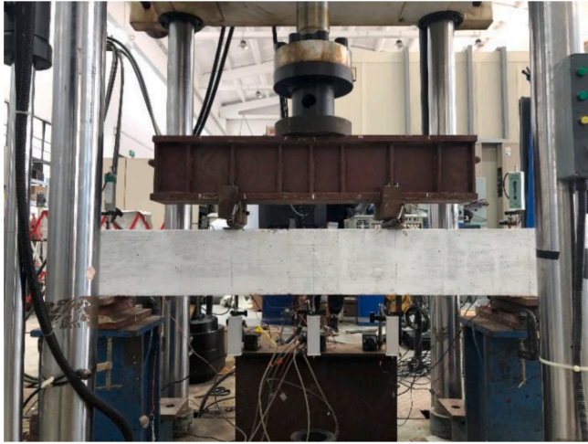
Fig. 5. Monotonic four-point loading of CFRP-strengthened RC beams.
