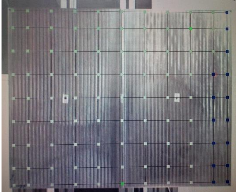
Figure 4. 7 : Grid which defines the scan points on the test structure
