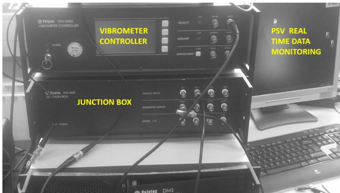
Figure 4. 2 : Assembly of Polytec controller, junction box, and the connected computer for real time monitoring of data
