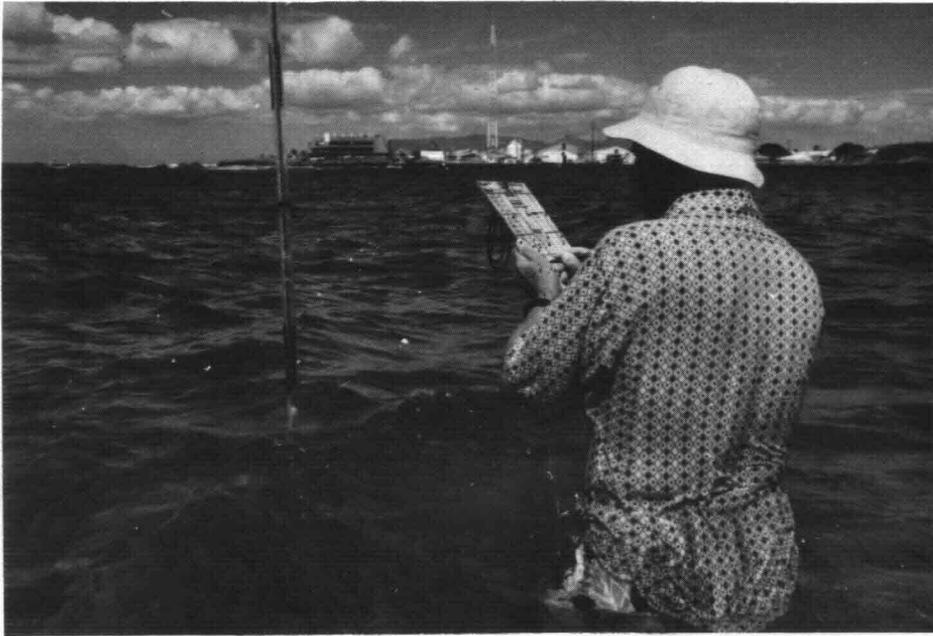
Figure 8.4-a Reading of Manometer for Wave Set-Up
