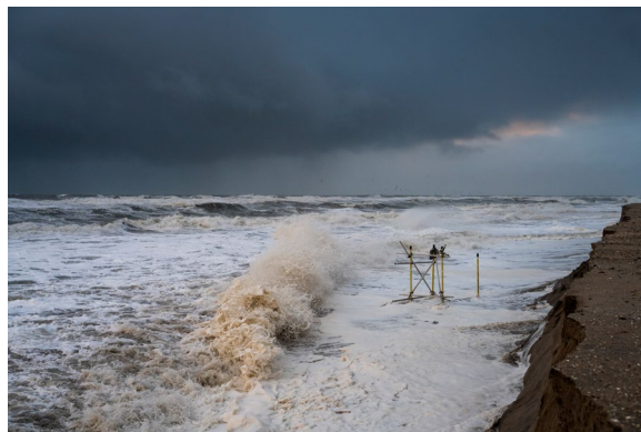
Fig. 1 Impression of dune erosion at Dune 1 of the field site (Fig. 2) during storm conditions on January 5, 2022 (Ph. Mischa Keijser). Instruments were attached to poles and frames in front of the dunes. A 2DV lidar scanner was installed on the frame in this photograph.
