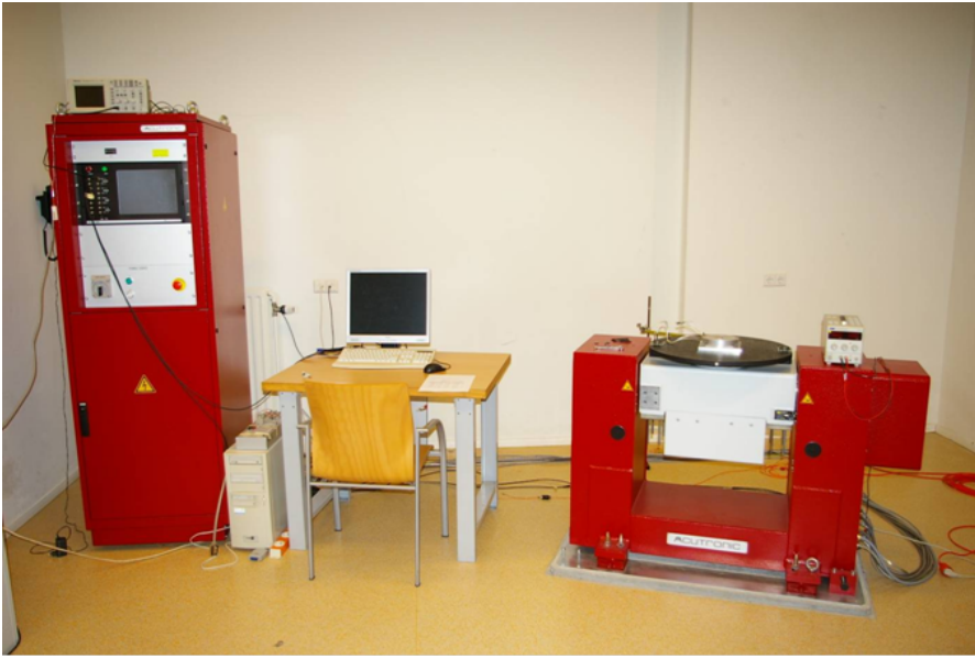
Figure 3.5: Picture of the gyro calibration on the rate table
