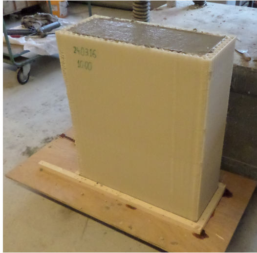
Figure 5-20: Casting of a built-up mould.
