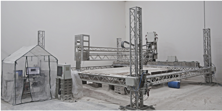
Figure 2-2: D-Shape binder-based printer (D-Shape, 2014).
