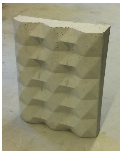
Figure 9-3: Case study: wall panel after demoulding.
