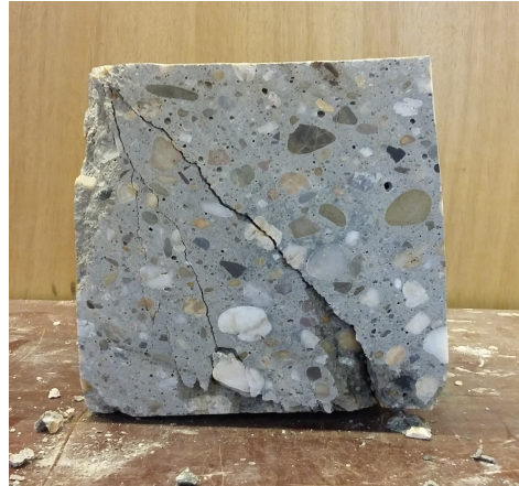
Figure 5-21: Concrete compressive strength test: crack pattern.
