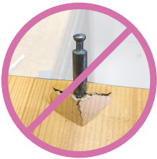
the classic cam-lock connection does irreparable damage
