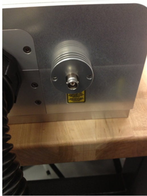
Figure 12: Externally mounted connector for internal photodiode on certain Nd:YLF laser models
