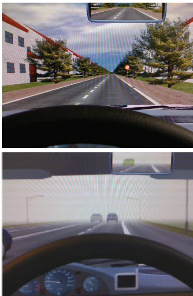
Figure 3.8: Test drive (top) and experimental condition (bottom) in the driving simulator.
