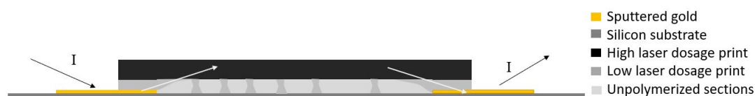
Figure 5.45: Electrical conductivity of microstructures printed on gold pads
