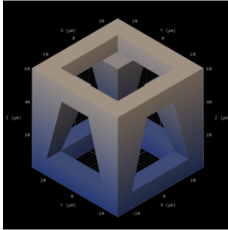
Figure B.14: Unit cell design with an inward angle on the pillar
