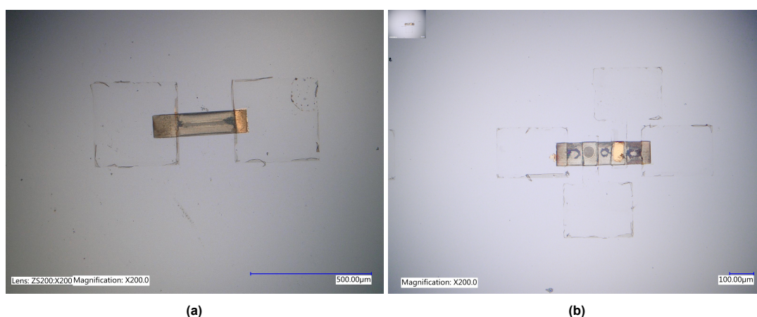
Figure 5.26: Delaminated gold pads for 5% doped microstructures, (a) 2-point probe, (b) 4-point probe
