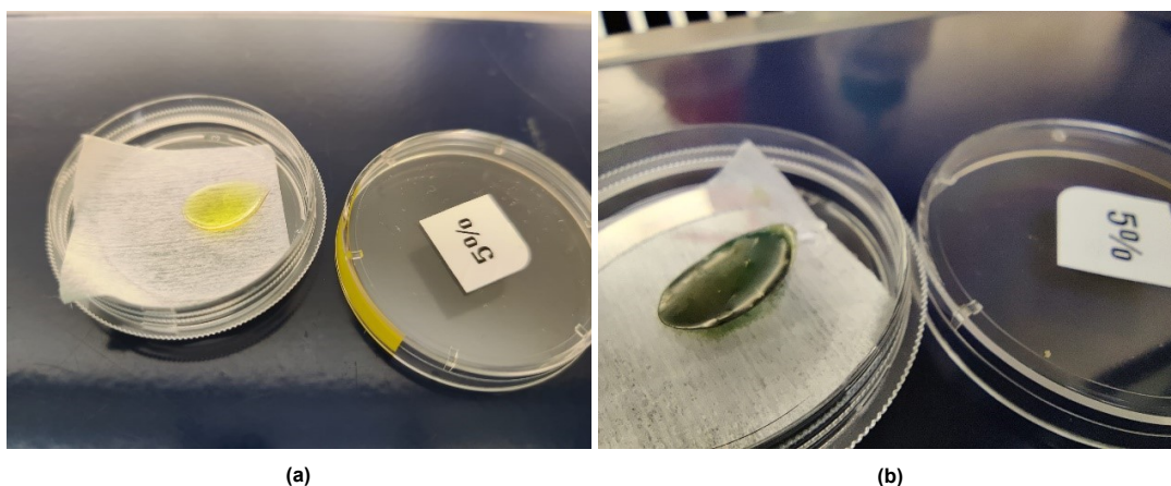
Figure C.1: (a)UV polymerized IP L EDOT 5%, (b) Oxidative polymerized IP-L PEDOT 5%
