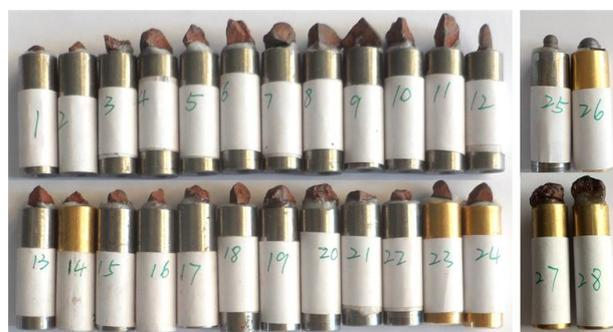
Fig. 6. Particle pins used for pin-on-disk wear test.
