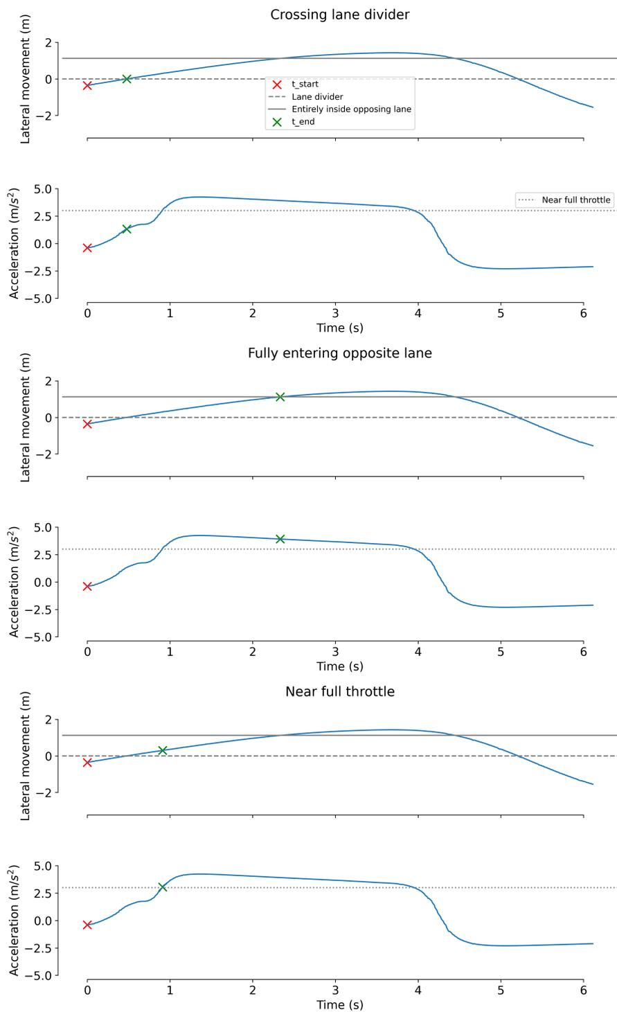
Figure 1.2: Comparison of response time measurement methods in accepted gap decisions, including the crossing lane-divider method proposed by Sevenster et al. [1] and two alternative approaches. Red and green crosses indicate the start and end of the decision-making process.
