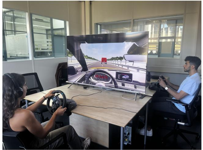
Figure 1: “Reverse” Wizard-of-Oz’ experimental setup of the driving simulator. During sessions involving oncoming human-driven vehicles, the experimenter operated an unconnected driving simulator setup.
