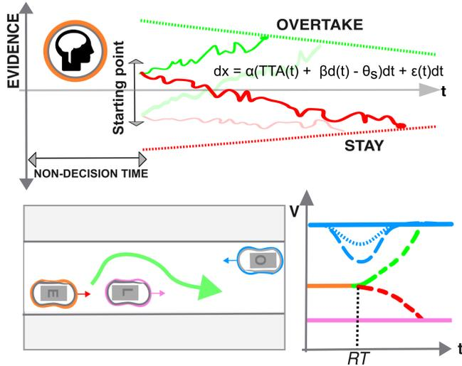
Figure 7: Gap acceptance visualization in overtaking scenarios using the drift-diffusion model. Purple represents the lead vehicle, blue is the oncoming vehicle, and orange characterizes the ego vehicle’s human driver. Red indicates staying in the lane, and green represents overtaking, while blue velocity curves depict different dynamics of the oncoming vehicle.
