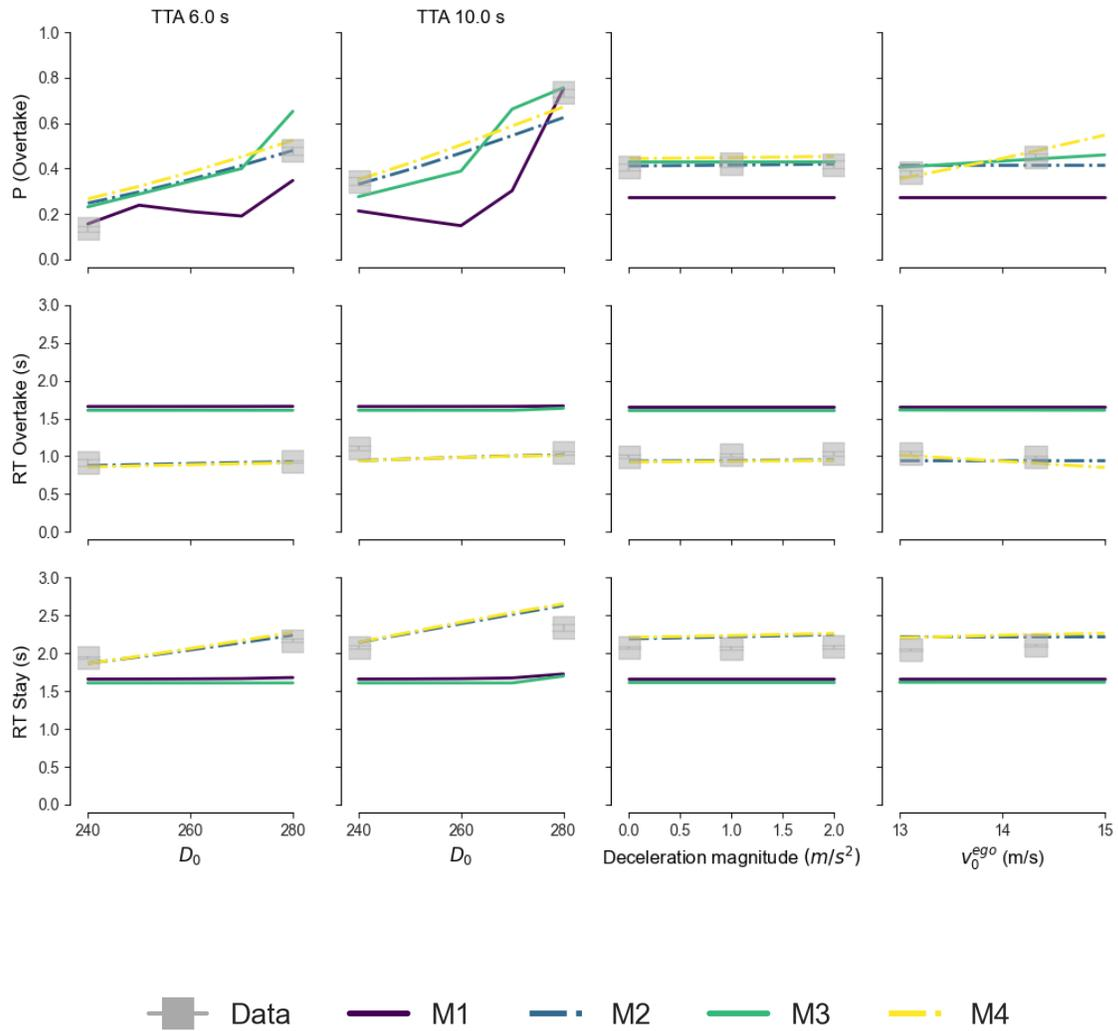
Figure 8: Simulated model results compared to the experimental data to show the effect of distance and TTA, deceleration magnitudes of acceleration profiles, and the initial ego-vehicle velocity on gap acceptance behavior. The error bars represent the standard error of the mean.
