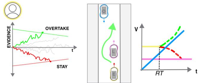
Fig. 1: Visualization of gap acceptance decision-making in overtaking. Depending on the gap to the oncoming vehicle (blue), the human driver of the ego vehicle (yellow) can decide either to reject the gap and stay in the lane (red trajectory) or to accept the gap (green trajectory) and overtake the slow lead vehicle. According to the drift-diffusion model, this decision can be represented as bounded accumulation of noisy evidence over time.
