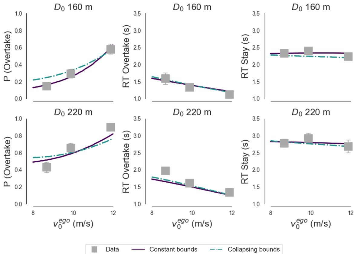
Figure 1.4: Simulated results of our model (Constant bounds) and Mohammad et al.'s [2] model (Collapsing bounds) compared to the data of Sevenster et al. [1]. The error bars represent the standard error of the mean.
