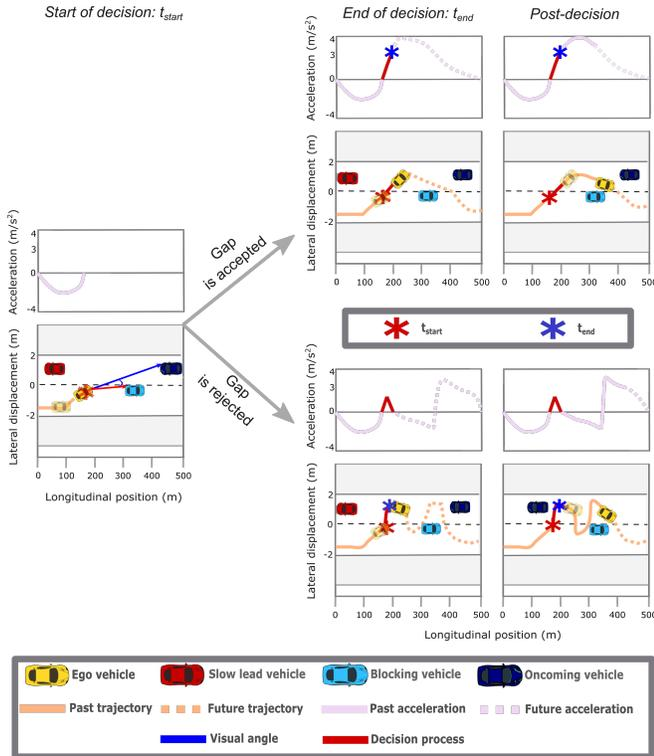
Figure 4: Response time measurement in rejected gaps [13] and our proposed measurement method in accepted gaps.
