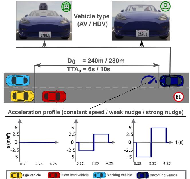
Figure 3: Experimental setup of the overtaking maneuver. The lead vehicle (red) slows down to induce an overtaking desire by the ego-vehicle (yellow). In each scenario, a distance and time-to-arrival gap to the oncoming vehicle (dark blue) is presented after the last platoon vehicle (cyan) passes. The oncoming vehicle, in half the cases an automated vehicle and in the other half a human-driven vehicle, drives with either of the three acceleration profiles.
