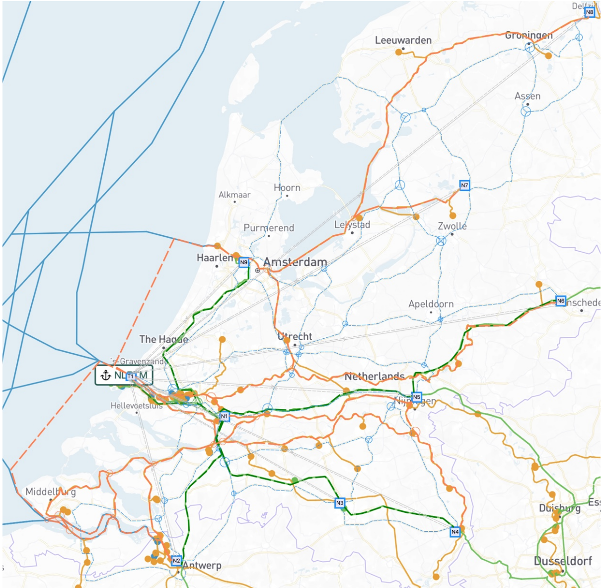
Figure 3.7: Hinterland transportation network in AnyLogic, based on existing routes from PoR Routeplanner.
