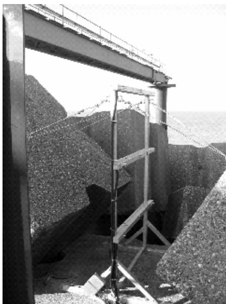
Figure 35: Velocity meter in front of dummy.
