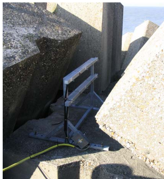
Figure 36: Velocity meter in front of pipeline.
