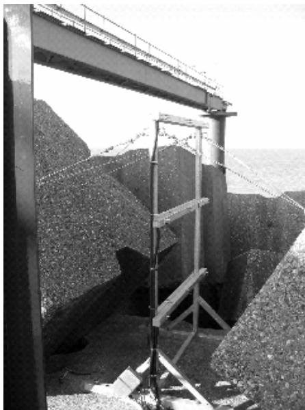
Figure 35: Velocity meter in front of dummy.
