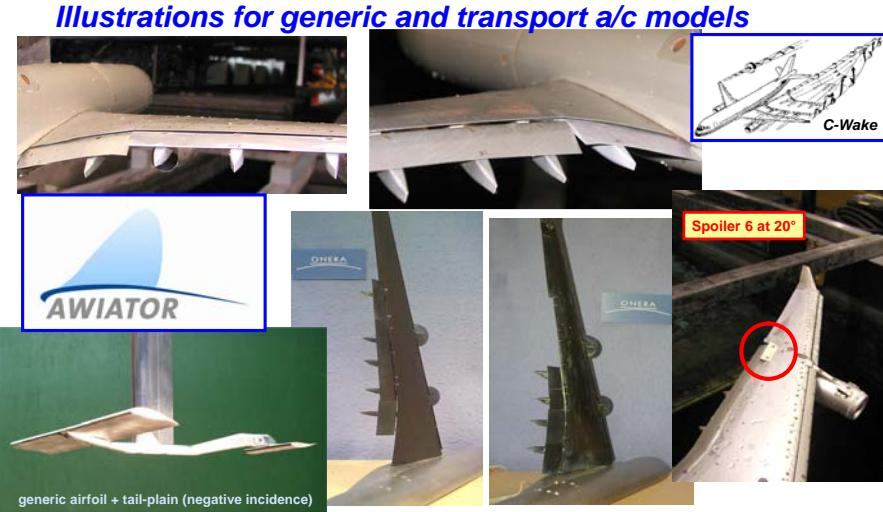
Figure 12 – Illustration of Differential Flap Setting “D.F.S.” concepts for 2- and 3-flaps high lift systems, and generic airfoil for generating four-vortex system.
