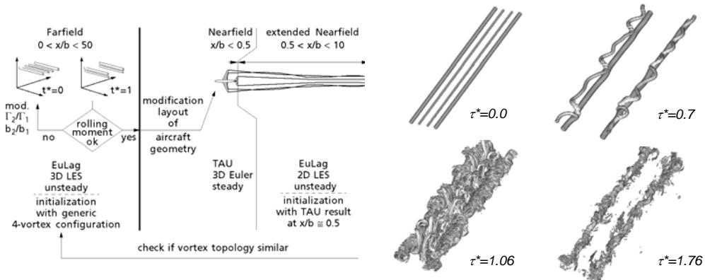
Figure 11 - Strategy for effective 4-vortex determination - left): numerical strategy; right): temporal development of iso-surfaces of vorticity for a given configuration [29].
