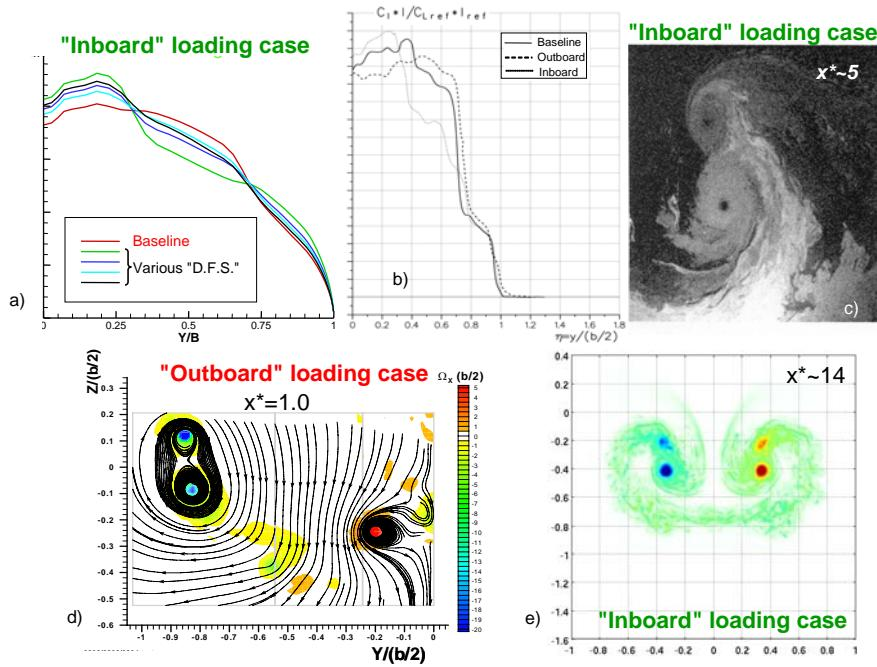
Figure 13 – Spanwise wing loading modifications for “Large transport aircraft-type model: a) computed load distribution [38]; b) load distribution deduced from measurements in the near-wake [24]; c) tomoscopy of the wake flow field [4]; d) measured wake flow field at  $x^* = 1$  [5,38]; e) computed wake flow field at  $x^* \sim 14$  [30,31].
