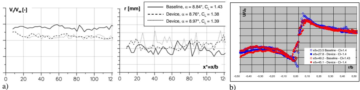
Figure 8. – Characterisation of wing add-on device (delta-type plate): a) peak vortex velocity and core radius (HSVA towing tank, PIV meas. [24]); b) tangential velocity profiles (B20 Catapult, Lidar measurements [3,24]).
