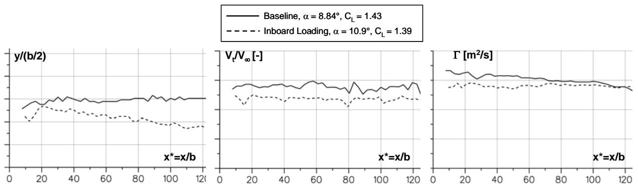
Figure 14 – Towing tank PIV results for inboard loading case on vortex spacing, peak velocity and circulation [24].
