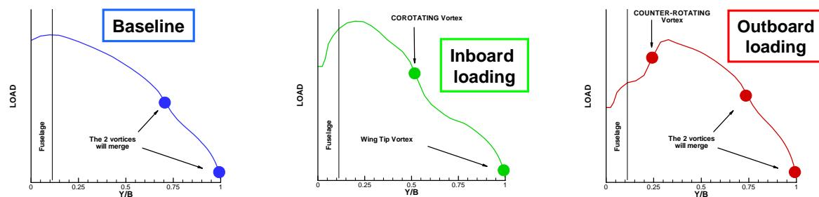
Figure 9 – Possible modifications of wing span load distribution ([38]).
