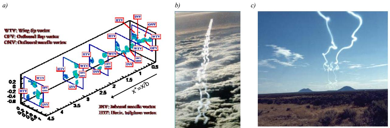
Figure 2 – Illustrations of wake flow fields a) Regions I & II: iso-contours of vorticity behind high-lift configurations (AWIATOR, exp. performed by TUM-AER [32]); b) & c) Regions III to IV (from [40]).
