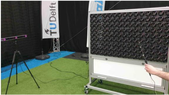
**Figure 2.22:** The multi-fan system of MAV Lab and the ProCap system [13]
