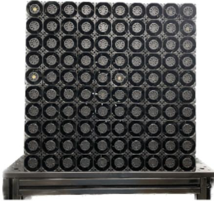
**Figure 2.25:** The small fan-array wind generator used in [33]
