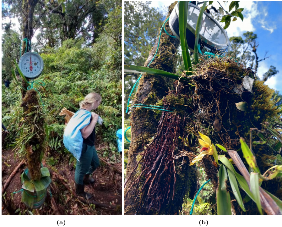
Figure 5.7: (a) Epiphyte Mass Interception and Evaporation estimation setup with gravimetric and volumetric measurements, (b) one of the orchids bloomed during our fieldwork.
