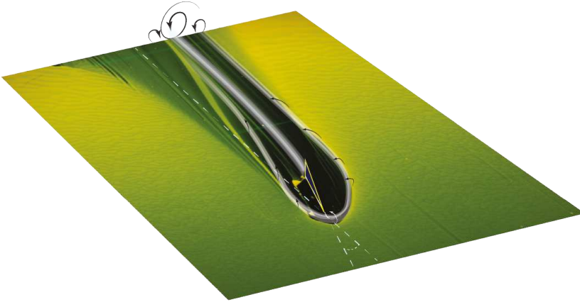
Figure 5.10: Flow visualisation of a singular embedded primary vortex, with expected associated secondary structures, depicted as bright streaks. Case: h = 10\text{mm} , x_{VG} = 20\%c , airfoil suction side, \alpha = 0^\circ in free transition.
