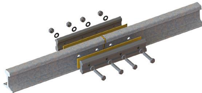
Figure 1.4: The IRJ and the parts it is made of (Quirchmair et al., 2020)
