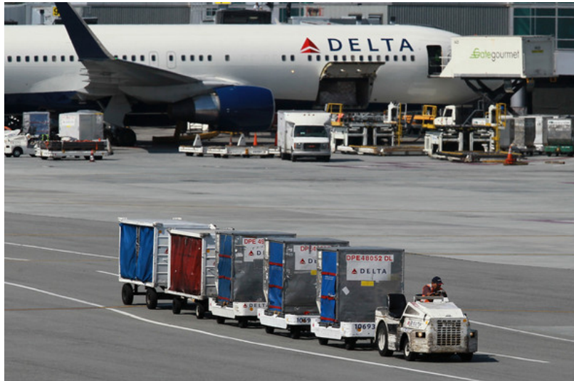
Figure E.4: A mixed train consisting of a tractor, three ULD carriers and two carts respectively for transport between make-up and aircraft [18].
