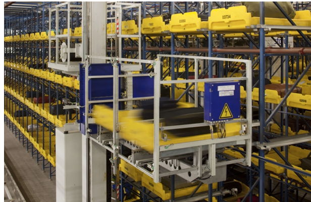
Figure E.12: Storage of baggage in an automated storage and retrieval system [24].
