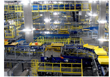
Figure 1.4: An ICS for the handling of baggage at Beijing Capital International Airport [4].
