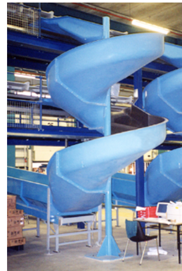
Figure E.5: Spiral chute that allows items to drop multiple levels [19].
