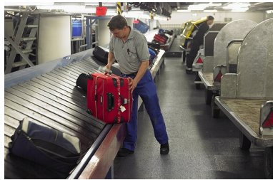
Figure E.7: Loading baggage carts from an inclined conveyor [20].
