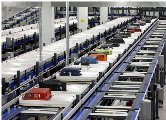
Figure E.11: Lane storage of baggage on an ICS at Bergen Airport [23].
