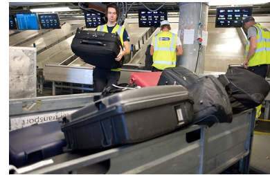
Figure E.8: Chutes collect baggage for a single destination [20].
