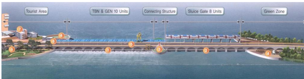
Figure 2.12: Impression of TPP Sihwa; Legend: 1-Turbines and generators; 2-Sluice gates; 3-Connecting structure; 4-Wing wall; 5-Road; 6-Tourist site; 7-Administration facilities; 8-Construction bay/ central control room.
