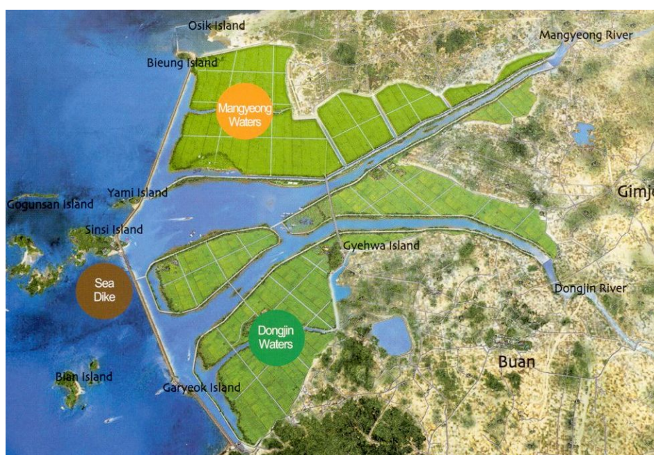
Figure 4.1: Layout proposed by KRC: fresh water reservoir of 117.6 km 2 and reclaimed tidal flats of 282.4 km 2
