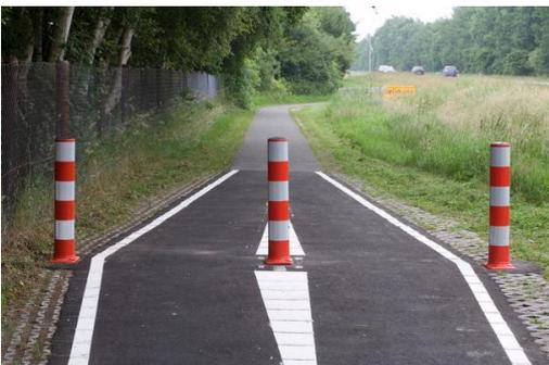
Figure 2.7: Implementation of a bollard according to the bicycle design guidelines (Fietsberaad, 2011)
