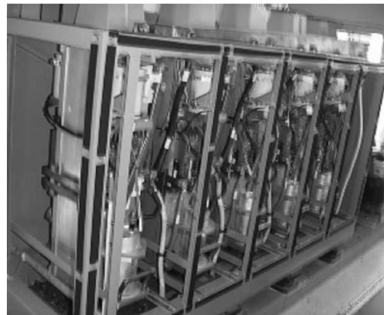
Fig. 8. Five inverters in parallel.
