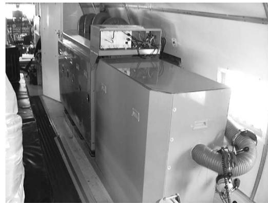
Fig. 7. Magnetic field transmitter unit in the fixed-wing aircraft.
