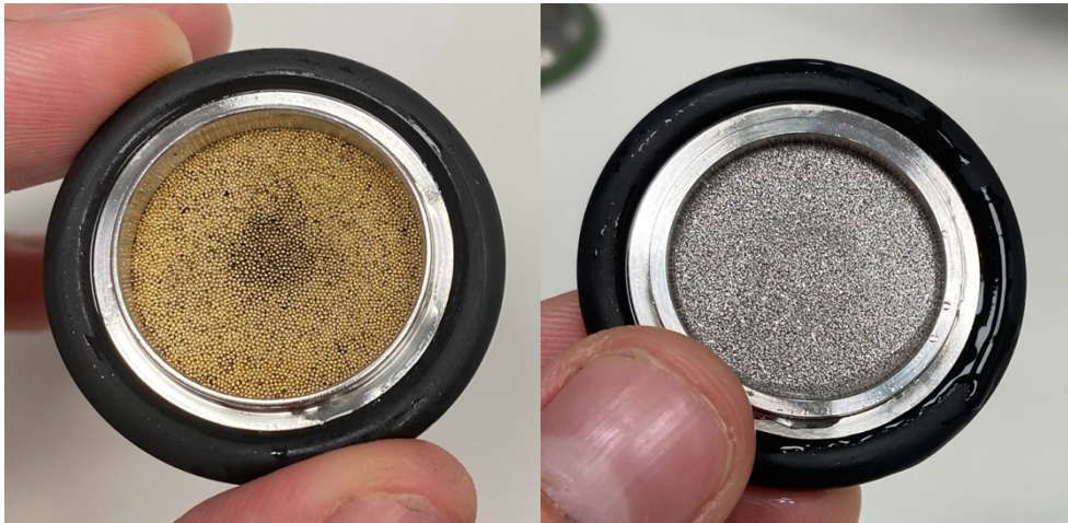
Figure 24 Porous tablets used in bubbling column: bronze (left) and stainless steel (right)
