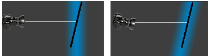
Figure 4.4: Using a tilt-shift lens allows the alignment of the Depth Of Field with the painting's surface. The Depth Of Field can be smaller when aligned, increasing the aperture and thus reducing the exposure time [90].
