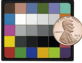
Fig. 6: The micro colour gauge chart with 30 colour patches used to calibrate the colour information.
