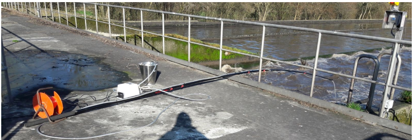
Figure 4.2: The used measuring set-up in action from the top of the oxidation ditch at WWTP Hattem
