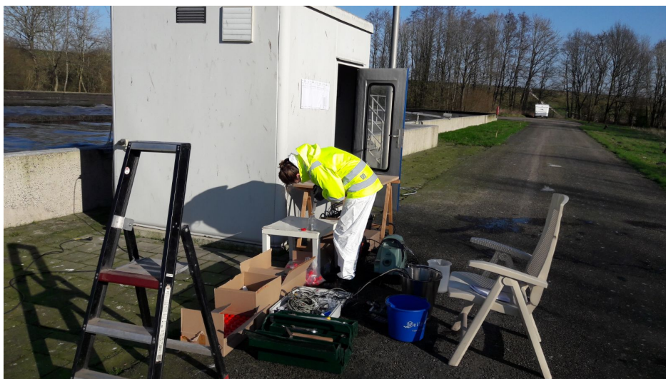
Figure 4.4: Filtering the samples next to the oxidation ditch
