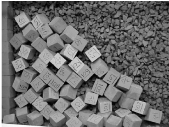
drop height 2.5 D_{\text{cube}} , placing density 72%
