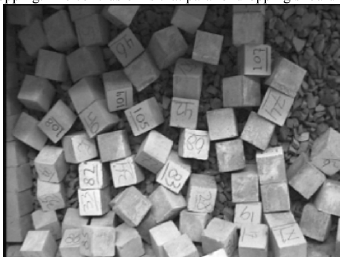
Figure 8: result of dropping blocks parallel to breakwater crest
