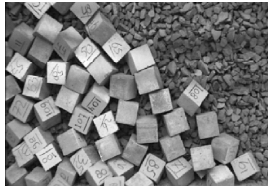
drop height 0, placing density 64%
