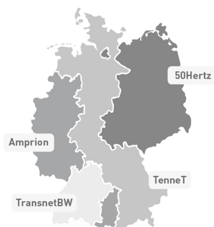
Figure 12 - German balancing zones and the respective responsible transmission system operators as per 2015 (Agora, 2015).
