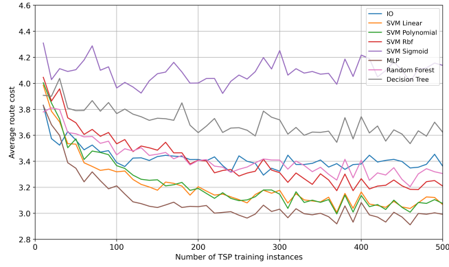
Figure E.1: TSP (random locations): Cost development during training using global policy training without feature vector transformation. Evaluated over 200 TSP test instances after each batch of 10 TSP training instances.
