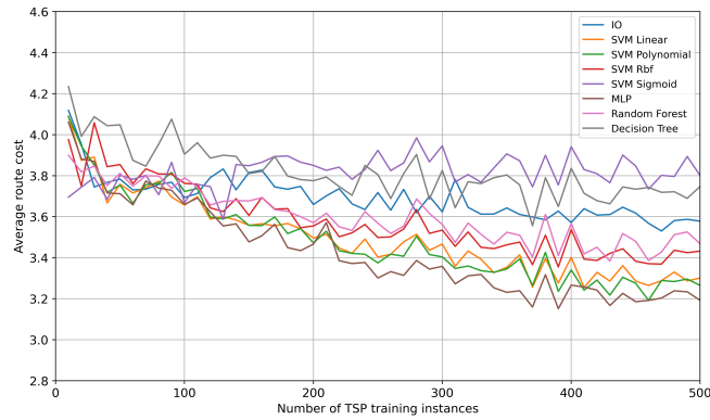
Figure E.3: TSP (random locations): Cost development during training using decisions policy training without feature vector transformation. Evaluated over 200 TSP test instances after each batch of 10 TSP training instances.
