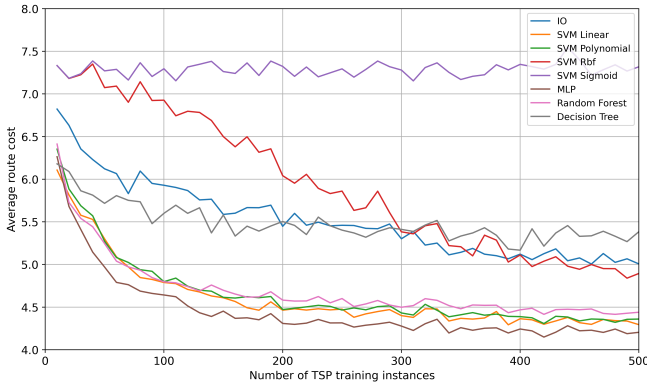
Figure 6.7: TSP (random locations, 20 nodes): Cost development during training using global policy training and feature vector reordering. Evaluated over 200 TSP test instances after each batch of 10 TSP training instances.
