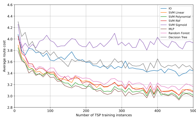
Figure E.7: TSP (random locations): Cost development during training using decisions policy training and feature vector reduction. Evaluated over 200 TSP test instances after each batch of 10 TSP training instances.
