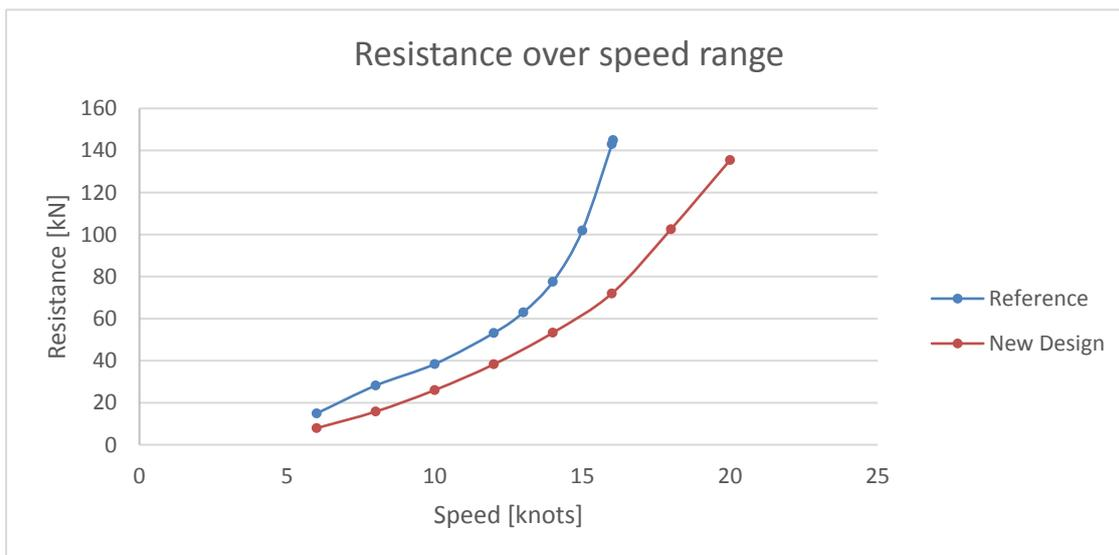
Figure 25: Resistance comparison between benchmark and new hull forms over the speed range
