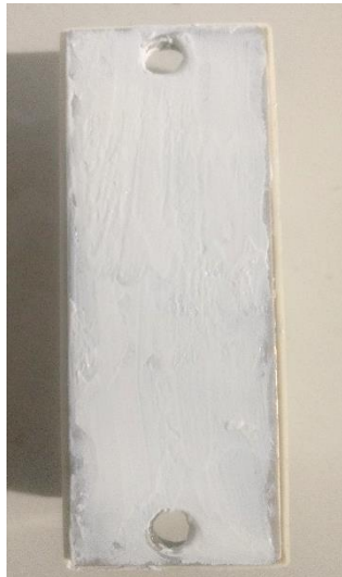
Figure 3.39: Thermal paste – before test
