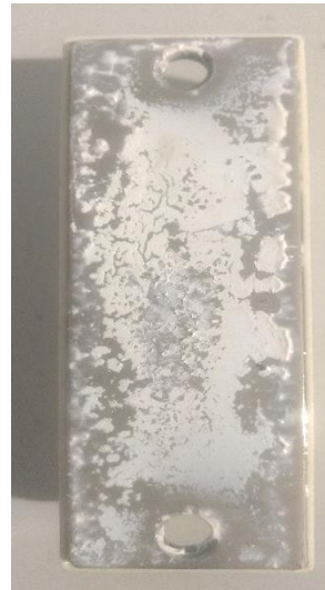
Figure 3.40: Thermal paste degradation – after test
