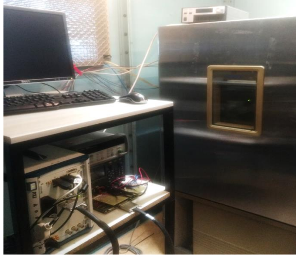
Figure 3.58: Entire test setup for the thermal cycling test
