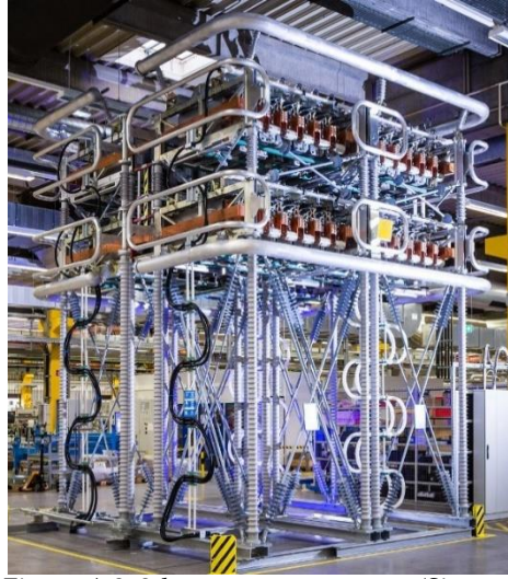
Figure A.3. 2-layer converter tower (Siemens) [83]
