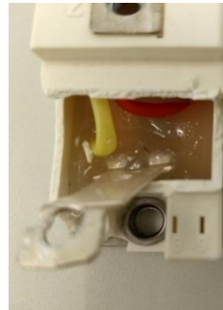
Figure 3.42: Image of the silicone gel inside tested IGBT module
