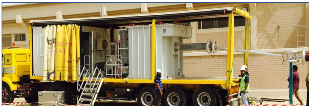
Figure 1.3: Internal view of the mobile test system manufactured by HIGHVOLT [8]
