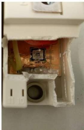
Figure 3.41: Image of the silicone gel inside the new IGBT module
