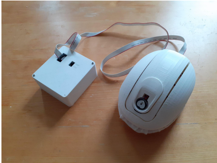
Figure 10: Prototype of Mini consisting of box with microcontroller and battery and separate unit with actuators and PPG sensor.
