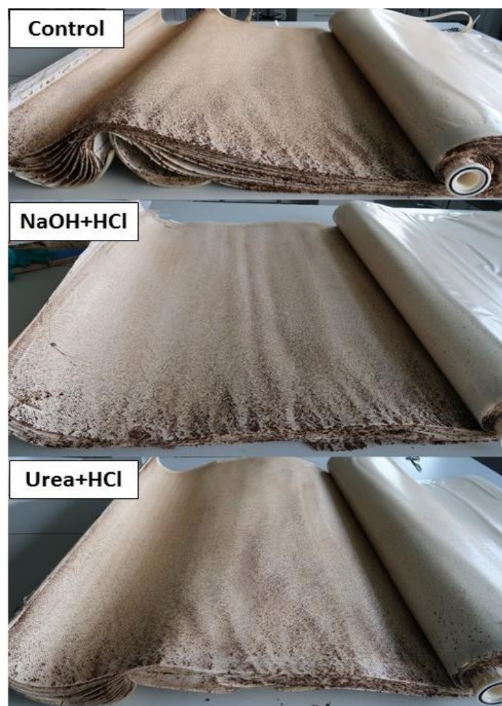
Figure 3. Visual comparison of the membrane/spacer surface of uncleaned (control) and cleaned membrane modules.
