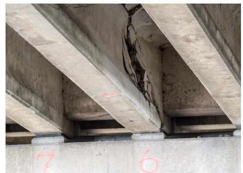
Figure 9 Punching failure deck test 1
