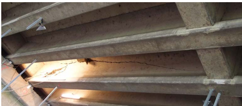
Figure 10 Shear failure beam test 2
