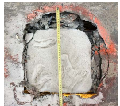
Figure 9 Punching failure deck test 1
