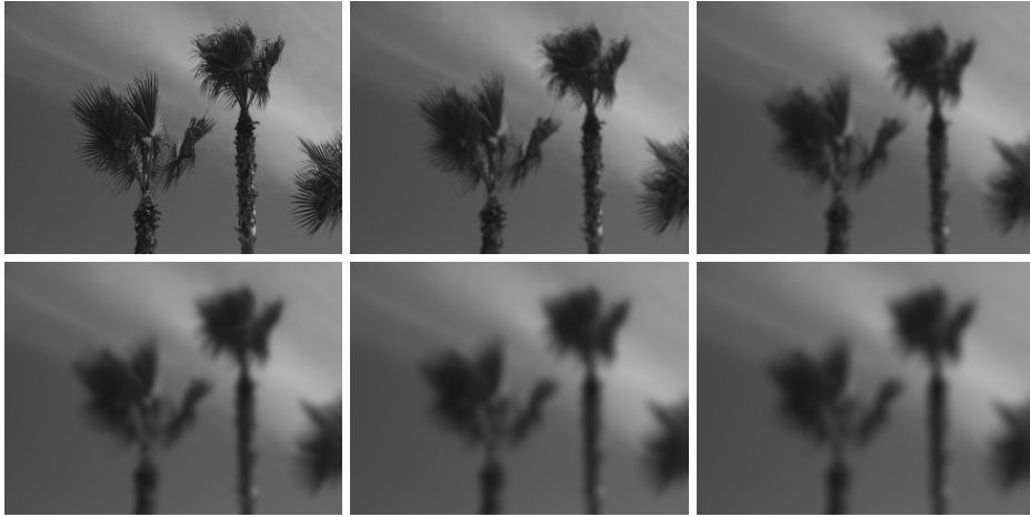
Figure 4.33: Images used for the reference measurements with different amounts of Gaussian blur. Top row: left: no blur, middle: \sigma = 1 , right: \sigma = 2 ; bottom row: left: \sigma = 3 , middle: \sigma = 4 , and right: \sigma = 5 .
