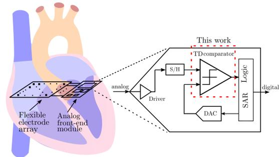
Fig. 1: System-level block diagram of a cardiac front-end
