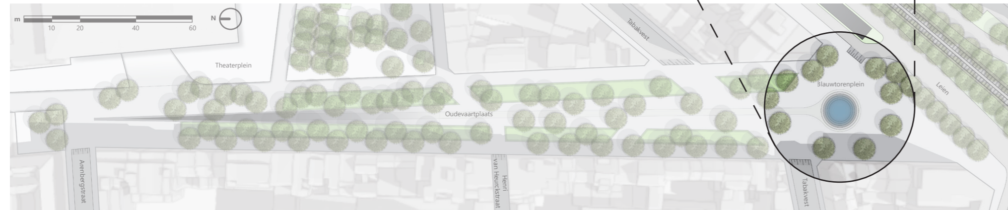
FIGURE 3.5.6: A zoom in plan view of the Blauwtorenplein shows how the fountain becomes an orientation point along the length of the street, attracting many spectators. The fountain acts as a cooling element to the public space and the steps of the pit can be used to sit on when the fountain is inactive. The view angle for figure 3.5.4 is also shown. (Own work).
