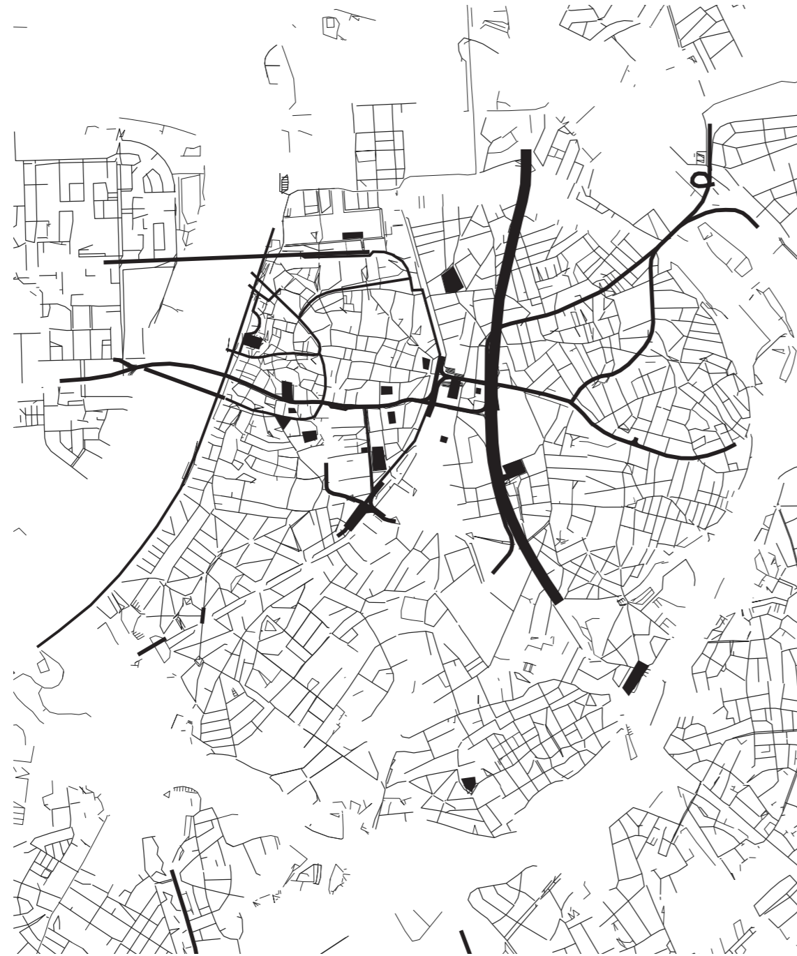
FIGURE 2.1.5: A figure ground map of the underground of the inner city of Antwerp (own work) shows what space is occupied (black) versus what space is not occupied (white). Occupied space mainly includes tunnels for cars, trains, and metros but also underground parking garages and a network of sewer pipes.
