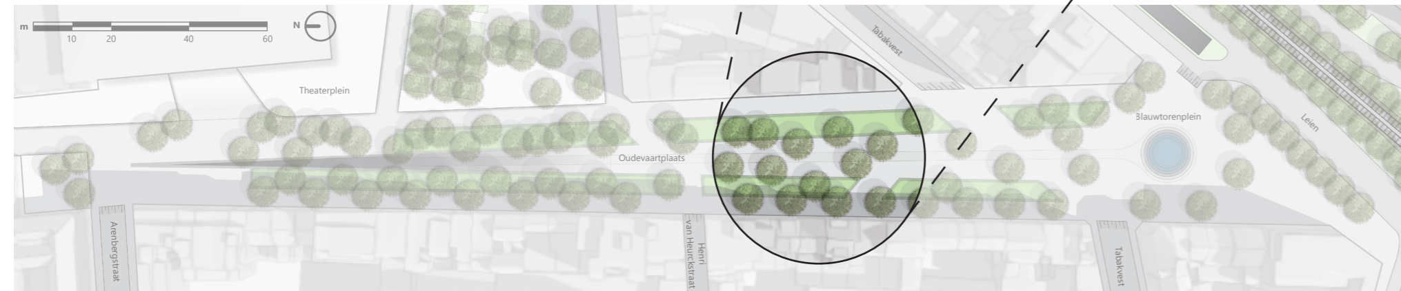
FIGURE 3.5.8: A zoom in plan view of the Oudevaartplaats shows how the parking space has made way for a linear square in which the market has more room. The helophyte beds beside the square act as an ecological buffer between the larger scale eco-capillaries along the Leien and the smaller scale eco-patches in the tunnel. The arrows show the flow direction of the water through the linear helophyte beds. The view angle for figure 3.5.7 is also shown. (Own work).
