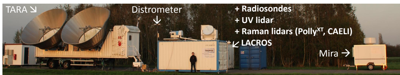
Figure 1. Measurement setup of the ACCEPT campaign at CESAR. The arrows point on the TARA radar (radar on the left), the disdrometer that is mounted on the LACROS container, and the vertical pointing Mira cloud radar (35 GHz). Complementary instruments of ACCEPT are listed but not visible on this photo.
